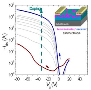
The effect of doping on the transistor performance of P3HT/PS blends and neat P3HT. In-situ evolution of the transfer characteristics ( $V_{ds}$ =-5V, linear regime) on exposure time in 'dilute air' (N<sub>2</sub> atmosphere with O<sub>2</sub> concentration ~1 ppm and H<sub>2</sub>O ~1 ppm). P3HT/PS (5% P3HT)
